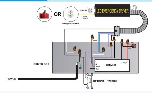
CAUTION: The voltage input to the dimmable wires (DIM+/DIM-) of the emergency LED driver must be less than 20Vdc.
